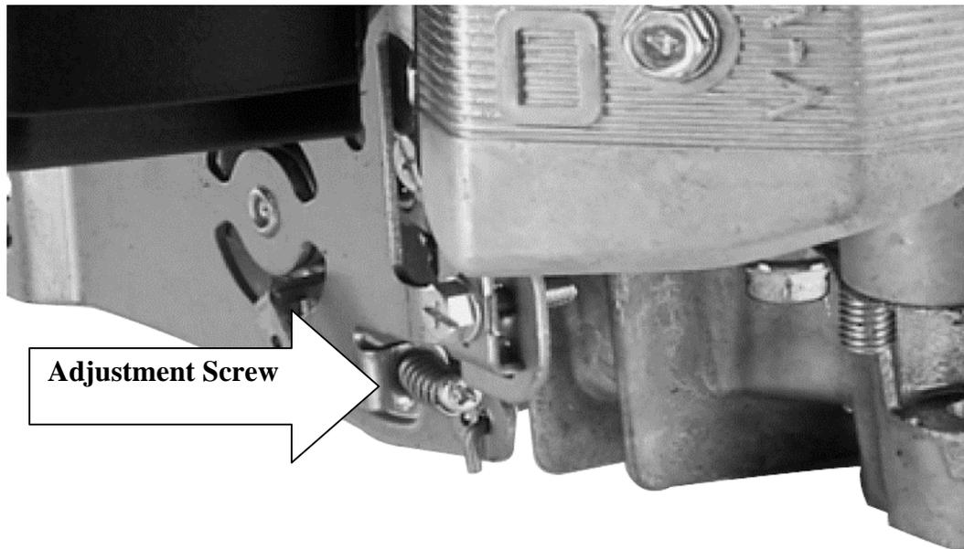
11. With the air filter removed, spray a little Gum Out, carburetor cleaner or starting fluid into carburetor. If engine fires briefly, check further for fuel problems such as the idle adjustment screw set incorrectly or clogged fuel line. If it doesn't check for electrical problems such as incorrect wiring, faulty fuel lock out or incorrect valve clearances.
